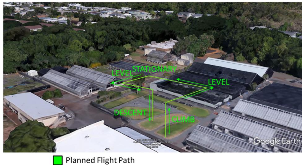
**Figure 8.** Planned flight path to evaluate flight stability and battery draw for validation flights.
