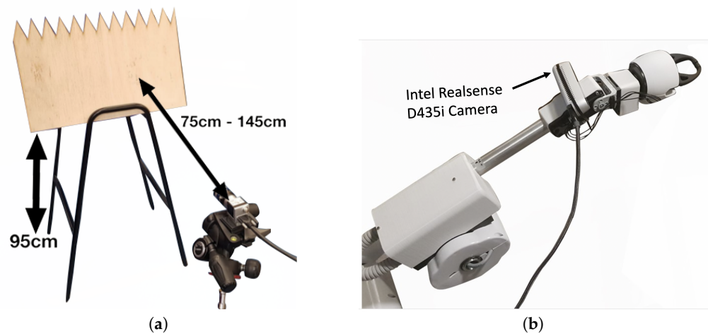
Figure 7. The lab setup for the environmental parameter experiments. (a) A photo of the environmental setup, showing the environmental parameter experiments. (b) A photo of the kinematic arm holding an Intel Realsense camera.
