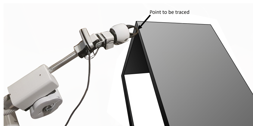
Figure 8. The tracing experimental setup with a hollow cardboard workpiece measuring 500 mm by 350 mm by 350 mm.
