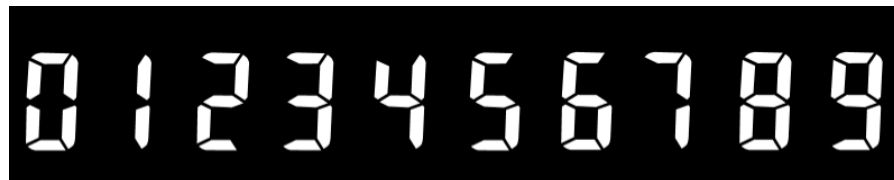
Figure 4. Reference template used for thermometer digit detection.
