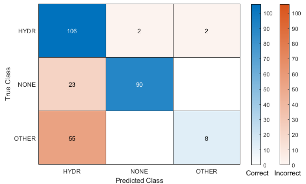
Figure 8. MC Dropout confusion matrix for test images.
