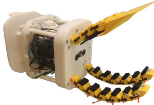
Figure 4. Underactuated gripper used to test the real application of the differential mechanism.
