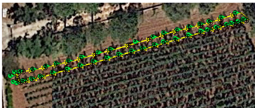
Figure 9. A typical pre-planned path in a vineyard. Green label: waypoints. Yellow line: interpolated path.
