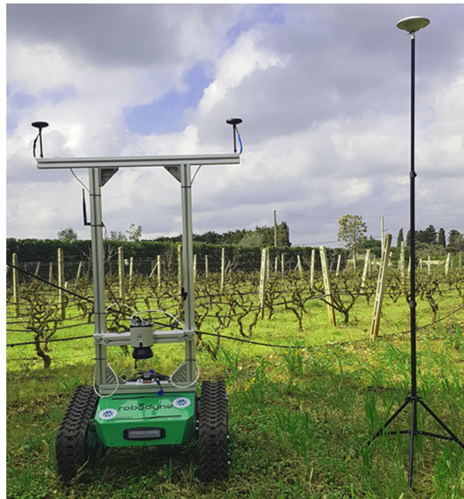
Figure 8. On the left, the vehicle with the dual GPS system. On the right, the base station antenna.
