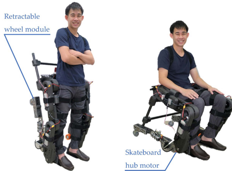
Figure 3. Alpha prototype of the wheelchair–exoskeleton hybrid robot in the standing upright posture (for walking across obstacles) and the wheelchair mode (for safe and low-energy traveling on smooth surfaces).
