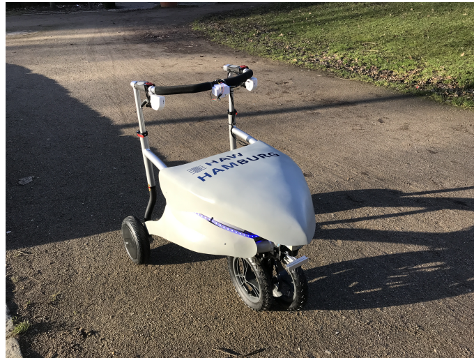
Figure 1. The Shared Guide Dog 4.0, an autonomous guidance vehicle resembling a rollator-walker.
