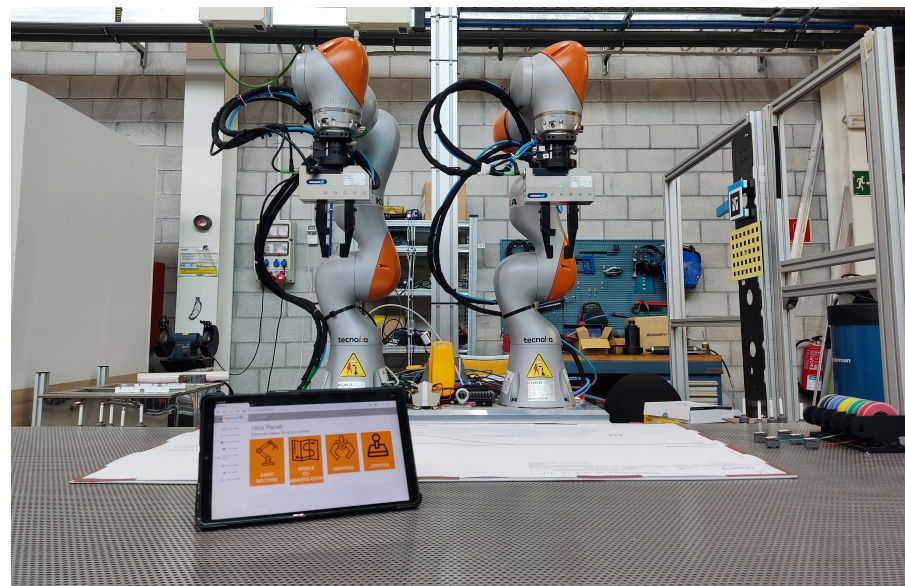
Figure 14. Robotic setup for wire harness manufacturing.
