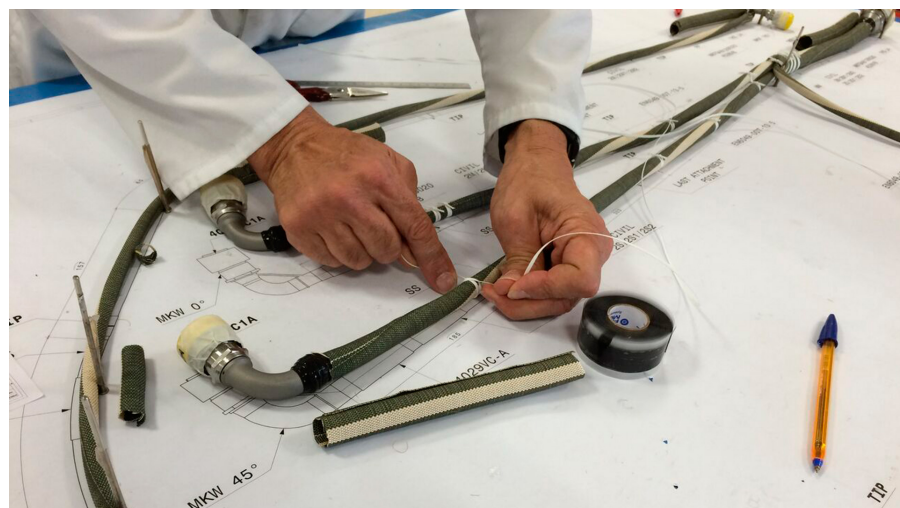
Figure 1. Operator working on the wire harness using the 2D drawing as a template.
