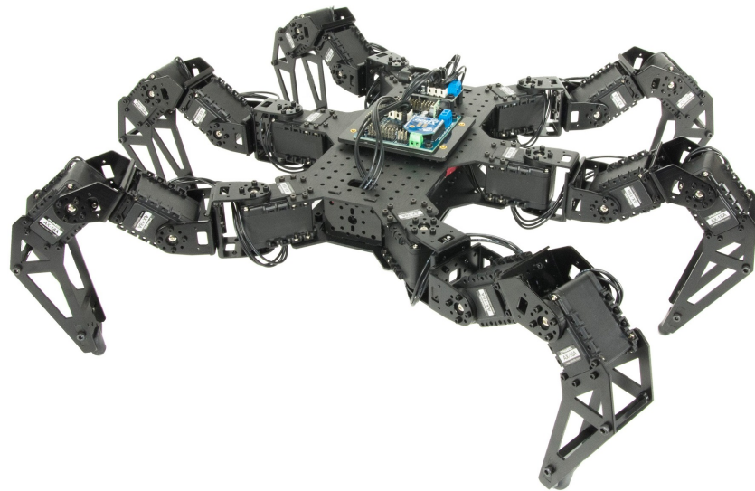
Figure 1. PhantomX AX Metal Hexapod Mark II [39].
