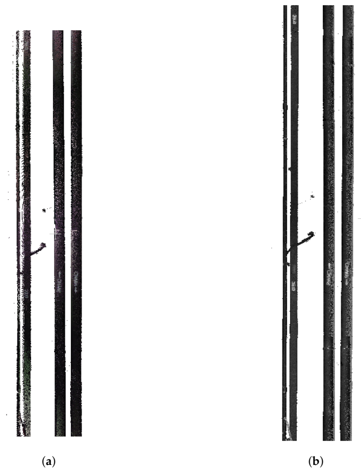
Figure 12. The top-down views of small portions of the MEP point clouds, as indicated by the light green boxes in Figure 11: (a) manual scanning results; (b) autoscanning results.
