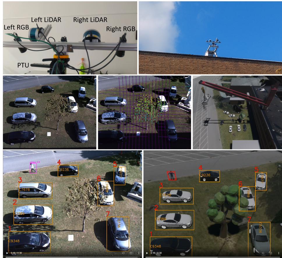
Figure 2. The first prototype of the 3DWI system for the rooftop recordings: The sensor suite on a pan-tilt unit ( top row ). The left camera view, projected LiDAR points, and the 3D-Twin of the rooftop environment and crane ( middle row ). The human activity detection and visualization in the 3D-Twin for the operator with corresponding object IDs ( bottom row ).
