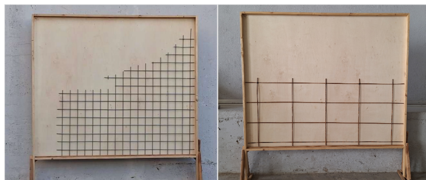
Figure 6. In the outdoor scene in Greece, the left image shows Testbed 01-a featuring a replica rebar structure, while the right image depicts Testbed 01-b with actual reinforcement bars used in building construction. Both rebars are installed in a custom wooden frame.
