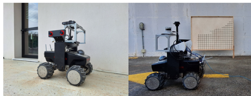
Figure 9. On the left: Robotnik Summit XL platform equipped with a Roboception RC-Visard 160 stereo camera mounted on the side. On the right: real-time testing of the integrated system during the experimental session in Testbed 01-a.
