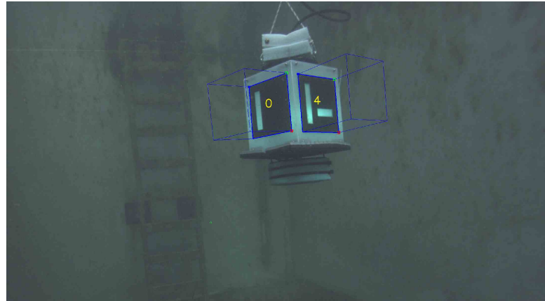
Figure 11. The ArUco markers, as detected by the ArUco detection algorithm.
