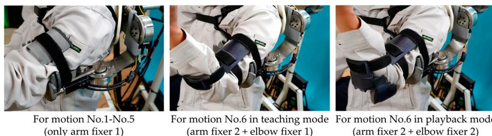
**Figure 9.** Combinations of arm fixer and elbow fixer in different cases.
