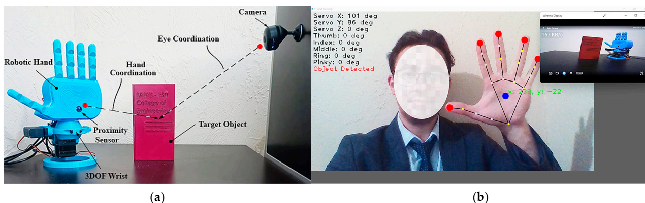
Figure 12. (a) Coordination framework of the novel bio-inspired 3DOF SRM for human–robot interaction. (b) Real-time hand tracking, object detection, and servo angle measurements for the bio-inspired 3DOF SRM.
