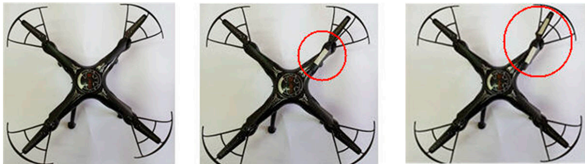
Figure 4. Three different blade configurations: balanced blade (at left), unbalanced blade with one strip of paper tape (at middle), and unbalanced blade with two strips of paper tape (at the right).
