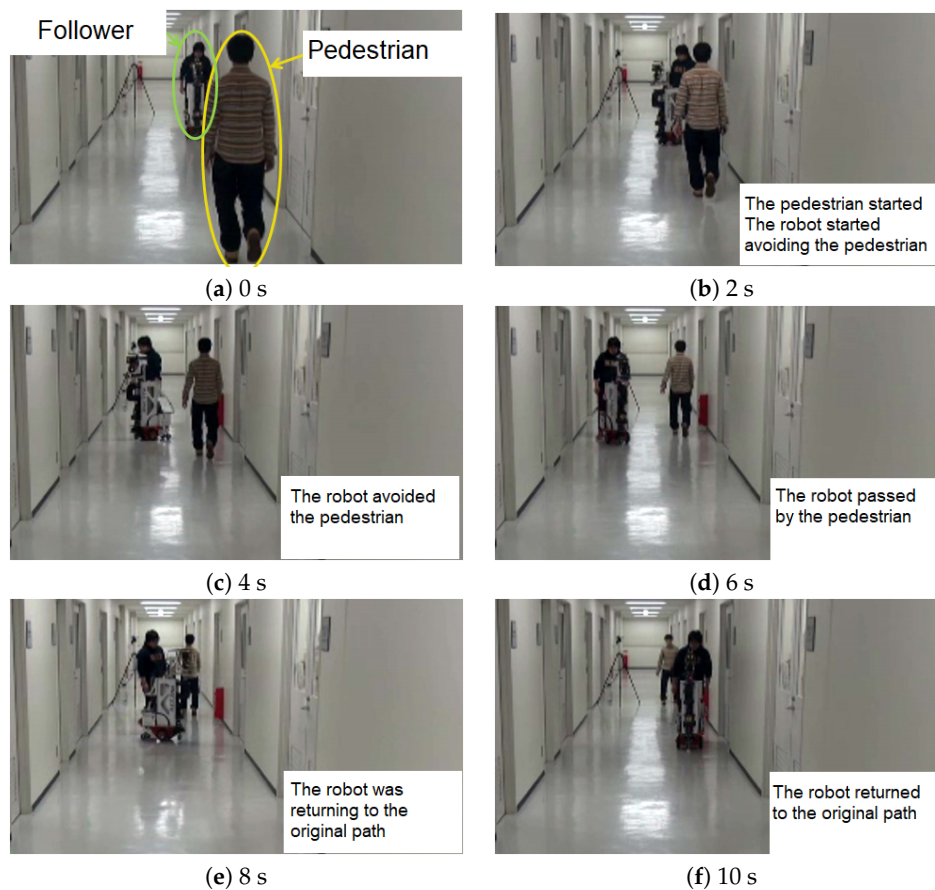
Figure 20. Photos of the experiment (trajectory \alpha , 1.4 m/s).
