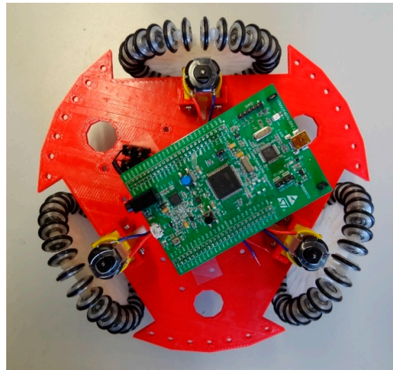
Figure 14. Top view prototype implementation of a compact mobile robot based on the omnidirectional wheel design proposed in this paper.
