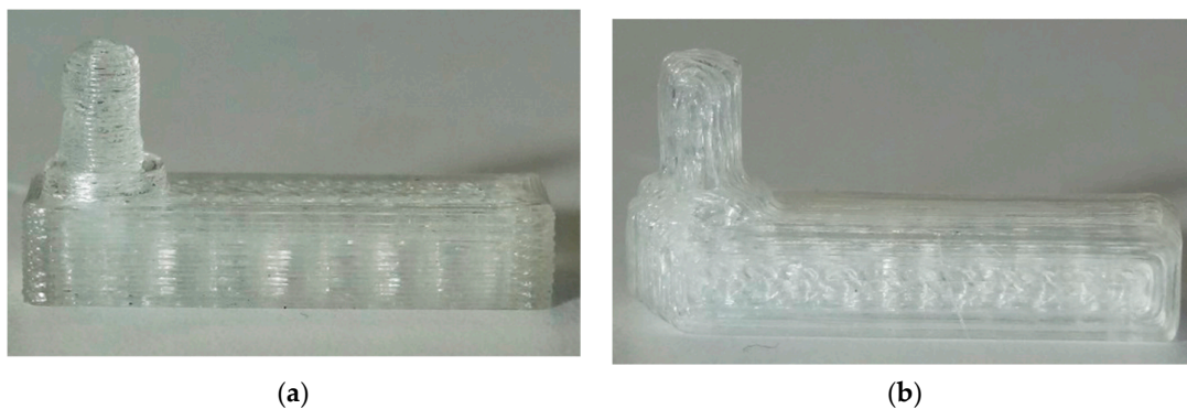
Figure 8. Detail of the successive layers conforming two half T-shaped structures printed with transparent polylactic acid (PLA) 3D850 (stick width of 4 mm): (a) printed vertically; (b) printed horizontally.
