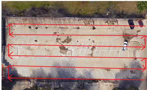
Figure 3. Grid flight pattern of UAV.
