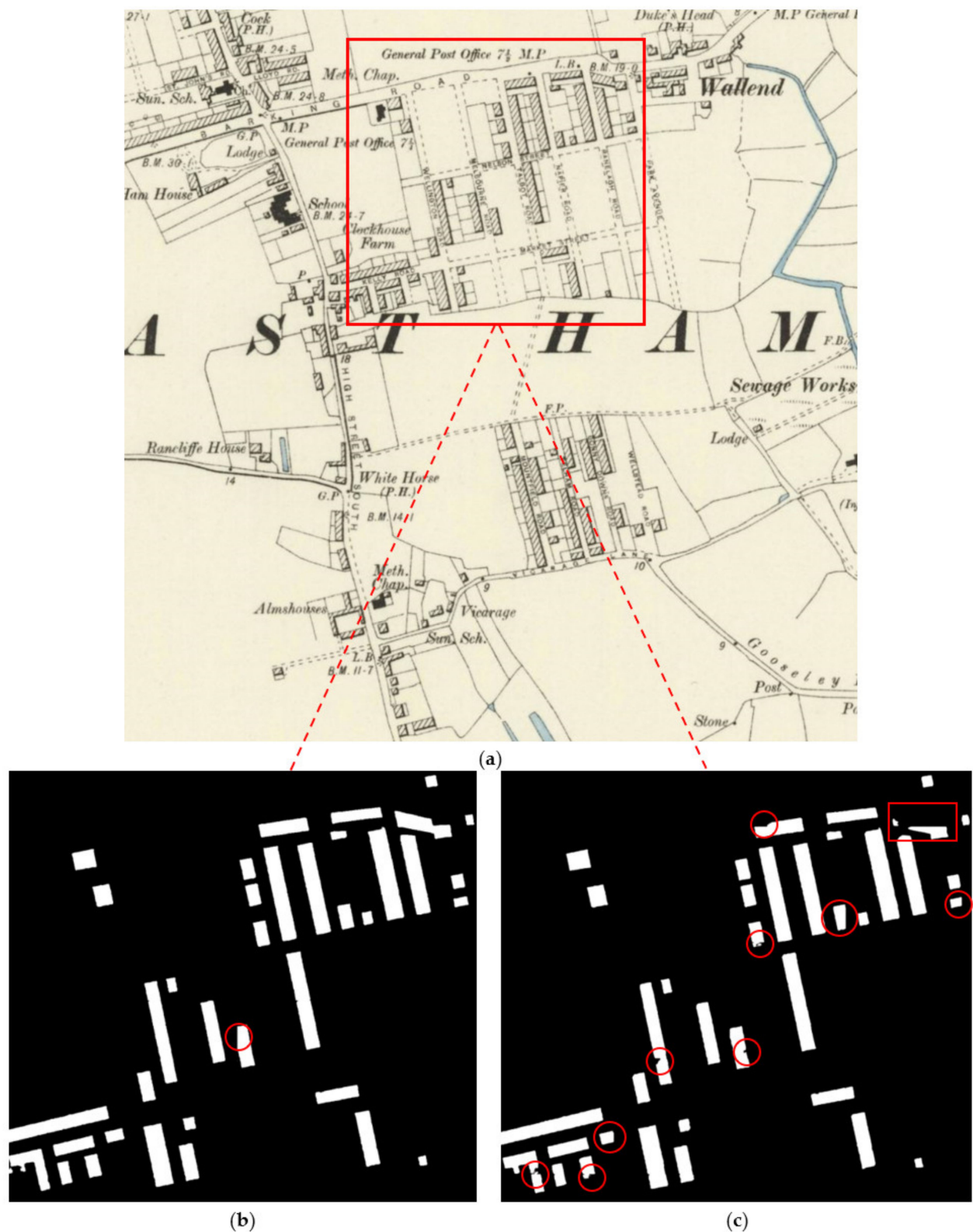
Figure 11. Comparison of extraction results with different numbers of segmentation tiles. (a) Experimental area; (b) identification result when the map image was cut into 16 tiles; (c) identification result when the map image was cut into 100 tiles.
