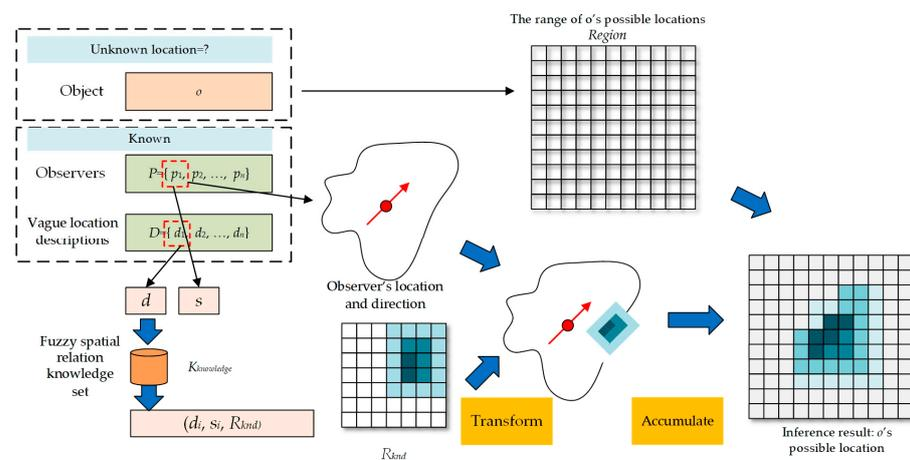
Figure 7. The inference process for extracting a spatial region from a description  $d$ .
