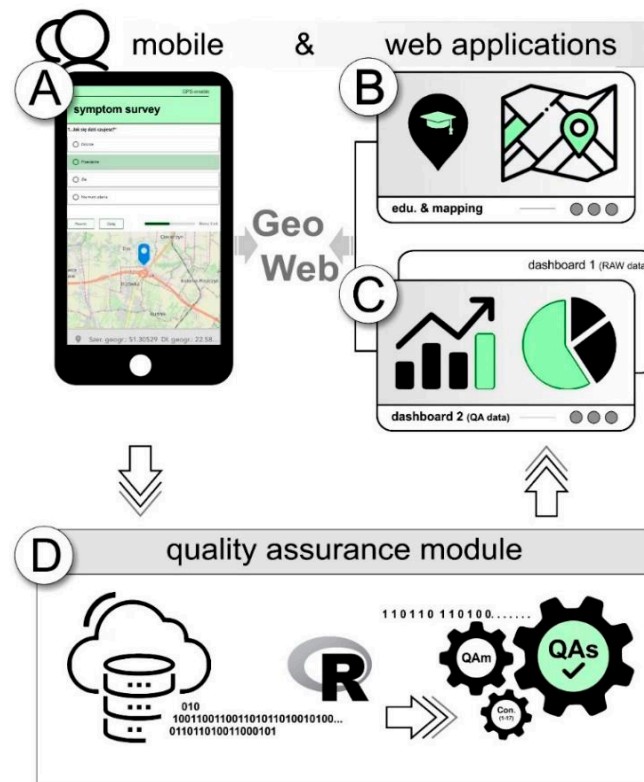
Figure 3. Geospatial web architecture implemented for the APSM project: (A) mobile survey app for field data collection, (B) web app with educational and training materials, (C) dashboard app for monitoring the data collection process and presenting APSM results, and (D) quality assurance module.
