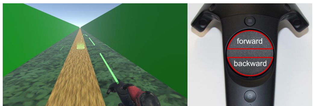
Figure 2. Implemented VR locomotion methods compared. The left side shows the teleportation function. Aiming with an arc that originated from the used controller allowed users to select a teleportation target. The right side demonstrates the controller assignment for the artificial locomotion. The upper 40% of the touchpad was assigned to a continuous forward movement, the lower 40% to a continuous backward movement.
