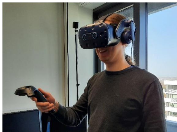
Figure 3. Used VR hardware. Participants were equipped with an HTC Vive Pro HMD and an HTC Vive Controller.
