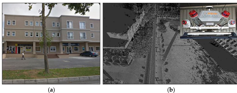
Figure 2. (a) ITU Yilmaz Akdoruk guest-house southern facade; (b) point cloud of the building facade and its environment measured by using the mobile laser scanning system (Riegl VMX-450).
