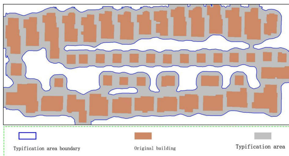
Figure 5. Construction of typification areas of buildings with the median filter.
