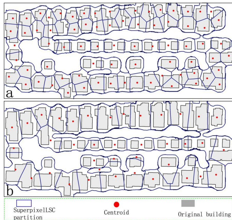
Figure 6. LSC superpixel segmentation is used to segment the typification areas of the building. (a) Small Aperture superpixel Blocking Results. (b) Big Aperture superpixel Blocking Results.
