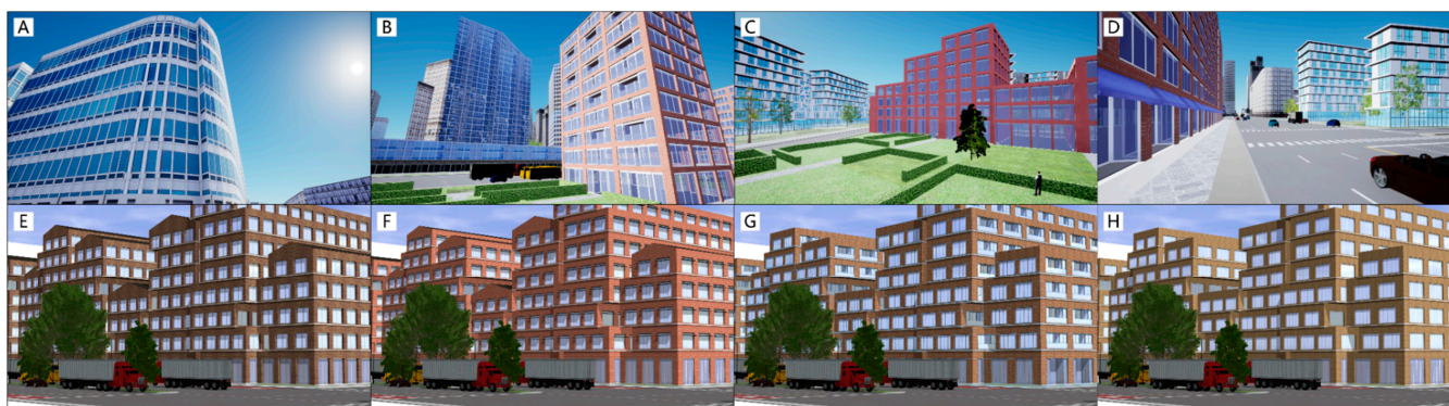
Figure 12. Different facade textures applied to the buildings ((A,B) showing textures for offices, (C) showing textures for schools, (D) showing textures for retail space, (E–H) showing different visual effects when applied certain textures in the same building, (E) applying double slope roofs and brown bricks on walls, (F) applying double slope roofs and brownish red ceramic plate curtain wall, (G) applying flat roofs and brown ceramic tiles on walls, (H) applying flat roofs and khaki bricks on walls).
