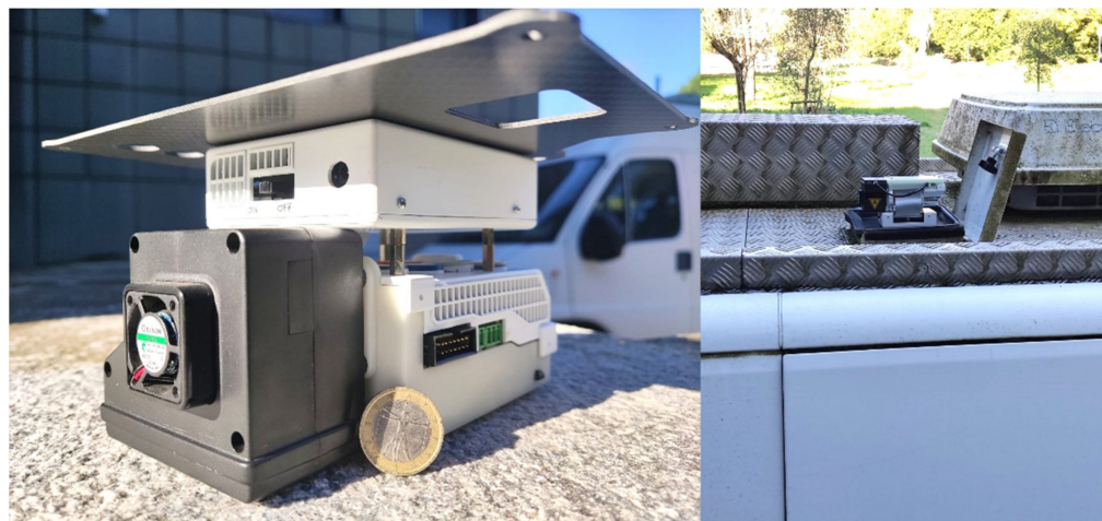
Figure 1. Air monitoring payload and its location on the roof of the van.
