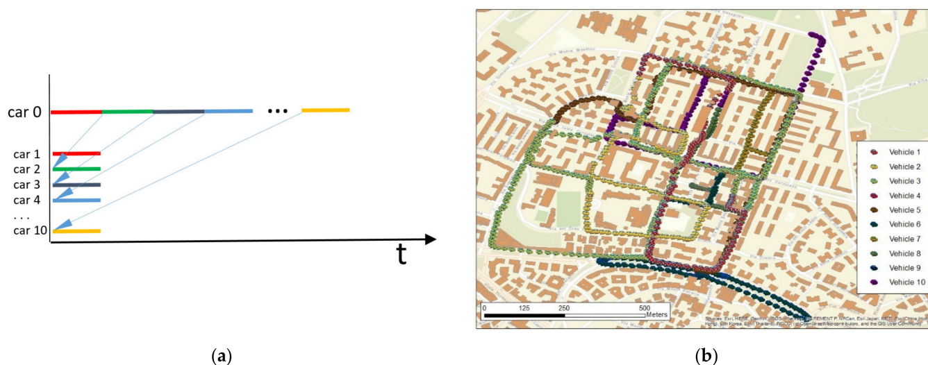
Figure 6. The experimental campaign: (a) the rearrangement of the data from a single recording to several smaller recordings; (b) the resulting location of data points on the map.
