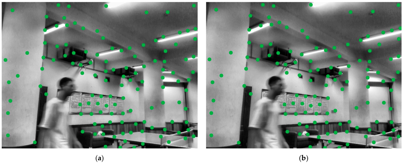
Figure 9. The results of feature point matching using the proposed algorithm. (a) Feature point distribution map of the previous frame image, and (b) feature point distribution map of the current frame image. Green points are static feature points.
