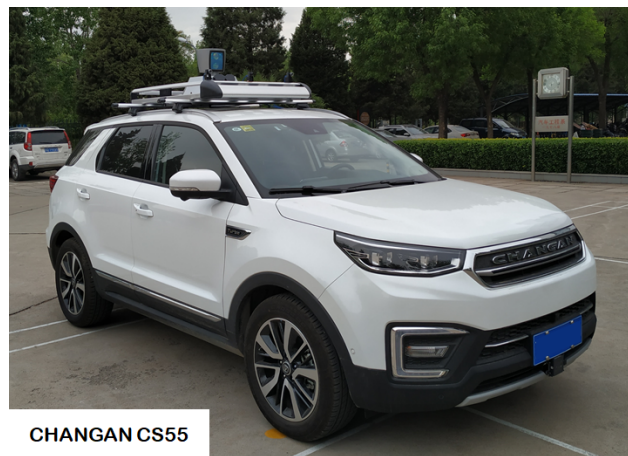
Figure 8. The vehicle used to collect the data for this experiment is equipped with the GNSS-RTK, IMU, monocular camera, and LiDAR sensor.
