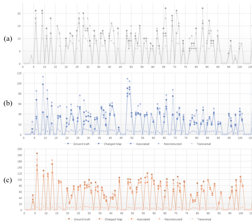
Figure 10. The number of map elements monitored during the vehicle transversals inside the linklet area: (a) traffic signs; (b) poles; (c) lane lines.
