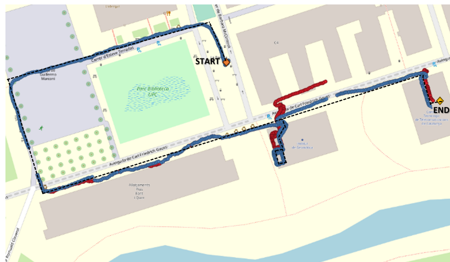
Figure 18. Comparison of the older seamless indoor–outdoor trajectory (red) with the newer one (blue) for the “PMT-LAB”. Ground truth trajectory is depicted in black (dashed line).
