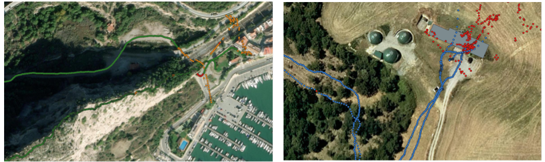
Figure 17. MK test applied to the trajectory of Falconera (left) and Colluspina (right). On the left figure, green points are good GNSS areas, orange are transitional areas from outdoor to indoor, and red are from indoor to outdoor. On the right, blue points are good GNSS areas while red points are indoor areas.
