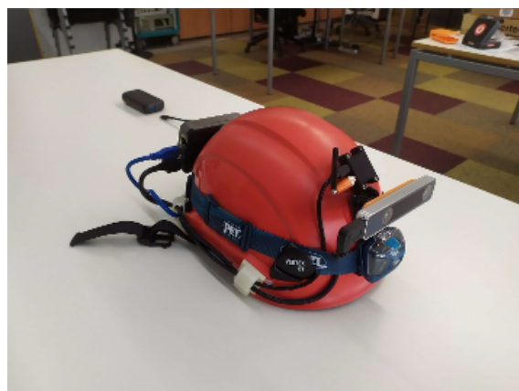
Figure 1. Positioning system mounted on a helmet designed and built by CTTC.
