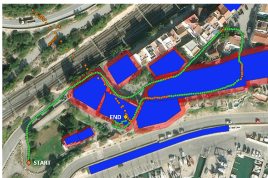
Figure 16. MK test applied to the trajectory in Garraf town. Green points are good GNSS areas, orange points are transitional areas from outdoor to indoor. Building layouts are shown in blue while transition or semi-outdoor area for the Garraf town is shown in red.
