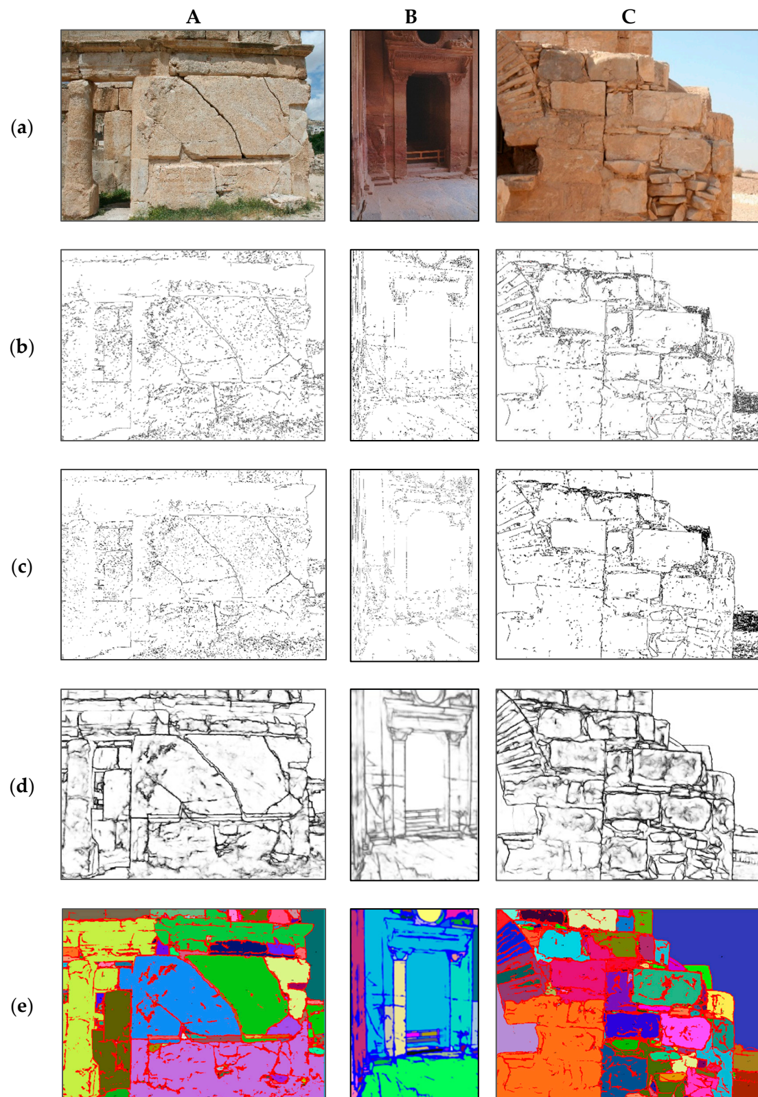
Figure 15. Experimental examples of feature extraction for building facades (A–C). (a) Original images. (b) Canny operator results. (c) Sobel operator results. (d) HED output. (e) HED segmentation.
