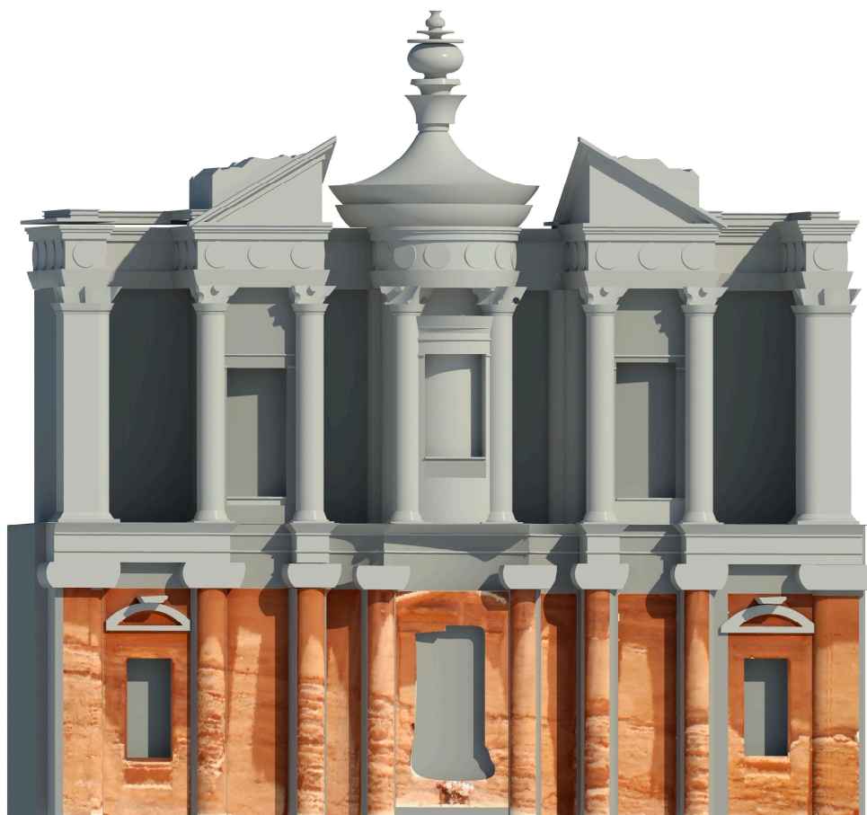
Figure 13. HBIM texturing using the produced true orthophoto.
