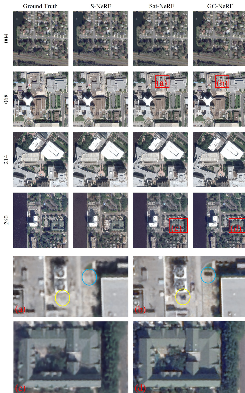
Figure 8. Images rendered by S-NeRFs, Sat-NeRFs, and GC-NeRFs. (a,b) Sat-NeRFs are robust to transient phenomenon such as cars. (c,d) GC-NeRFs render clearer images.
