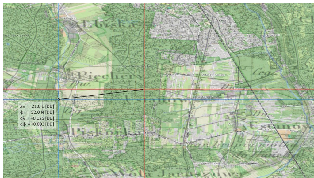
Figure 6. Location of the origin point of the coordinate system, i.e., the intersection of the Warsaw Meridian and the parallel 52 N on the TKKP sheet Col. 4 Sect. 4. (50% transparency). TKKP coordinates—red line, WGS 84 coordinates—blue line. Shift vector of the 10 min grid from point 21 E, 52 N to the origin point of the TKKP. OSM base map.
