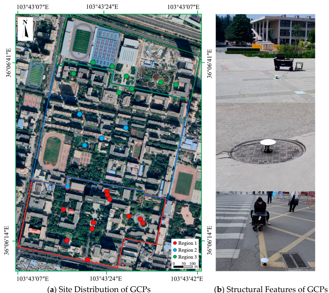
Figure 15. Location and Feature Selection GCPs for three regions in the Case Study Area.
