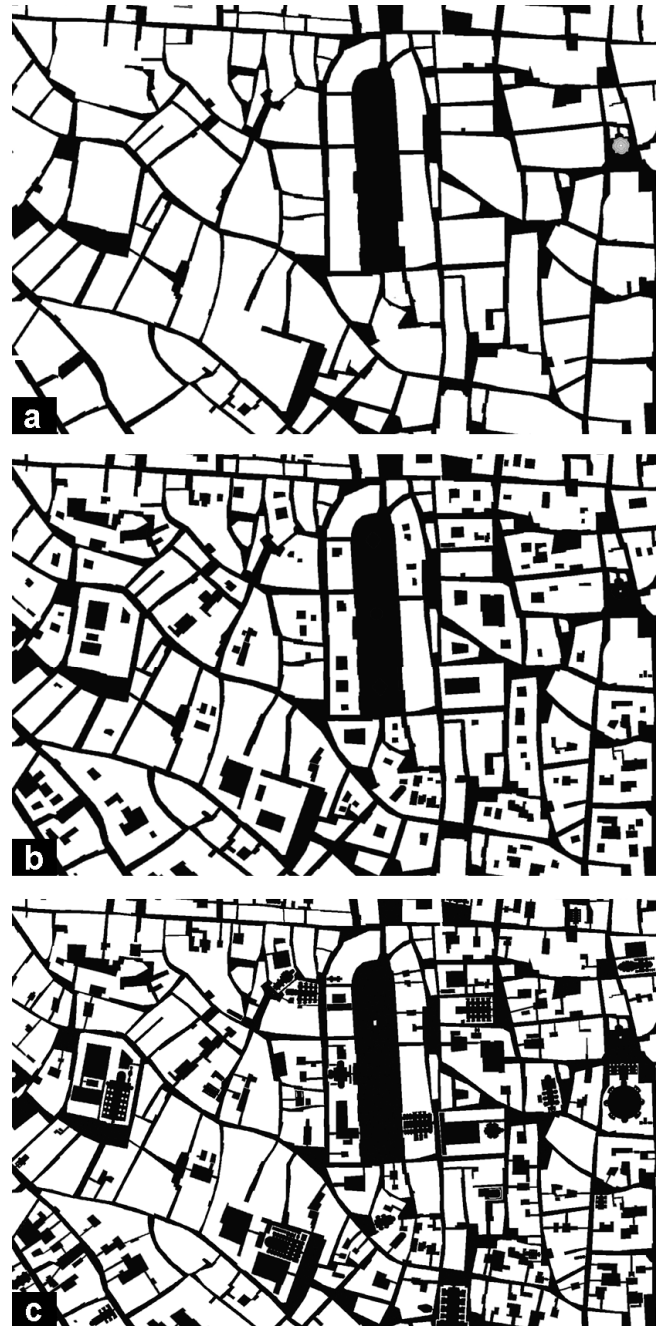
Figure 6. Vectorization of the Nuova pianta . Level of representation of the urban structure: (a) building blocks; (b) solids and voids; (c) including the plans of churches, noble palaces, arcades and covered passages.
