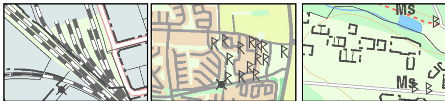
Figure 5. Maps that were often misclassified as readable: (left) maps with dense lines, (middle) maps with dense/overlapping symbols and (right) map with bad symbol types (of the cadastre boundaries).
