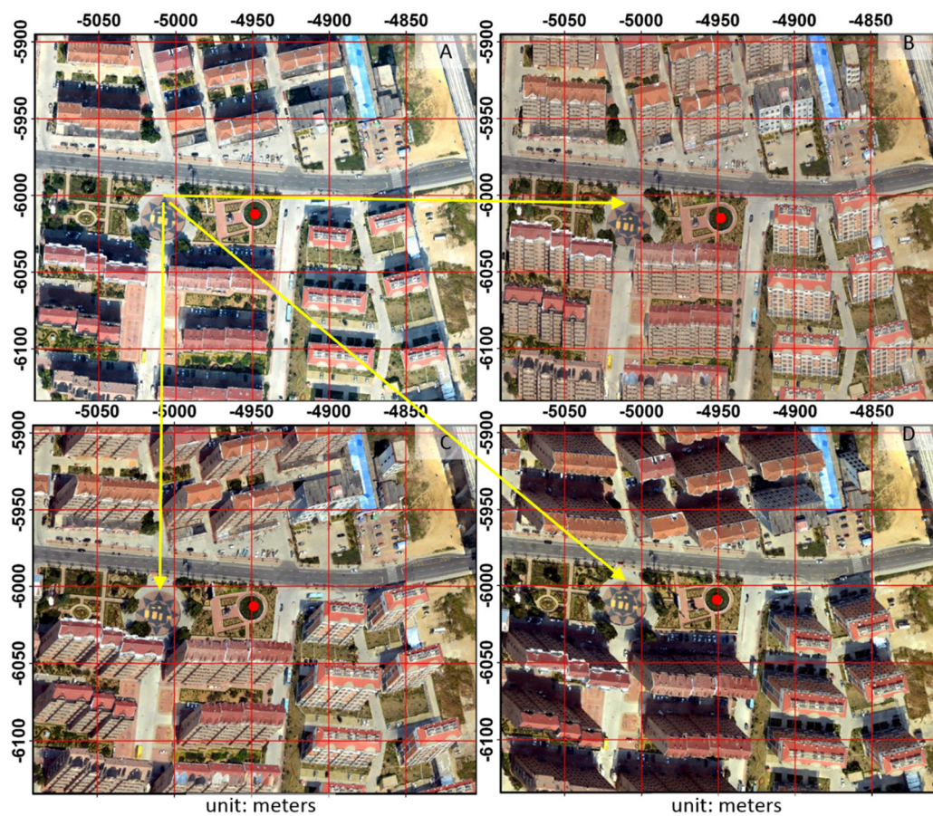
Figure 9. 2.5D maps of different perspectives created from Dataset 1 for assessing geometric accuracy (follow the yellow arrows to observe displacements): (A) orthographic view; (B) \theta = 0^\circ , \varphi = 45^\circ ; (C) \theta = 45^\circ , \varphi = 45^\circ ; (D) \theta = 135^\circ , \varphi = 45^\circ .
