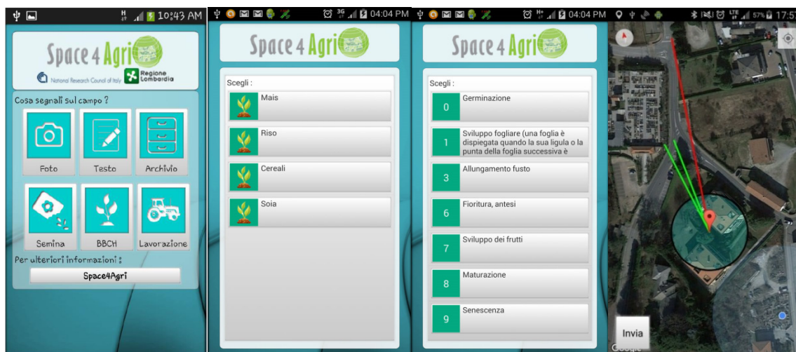
Figure 3. S4A smart app screenshots showing the main menu for VGI creation, the first and second level entries of the compact BBCH agronomic ontology and the representation of the GPS imprecision and camera orientation (depicted by the green line angle).
