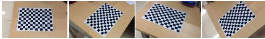
Figure 10. Four images of the model plane for camera calibration.
