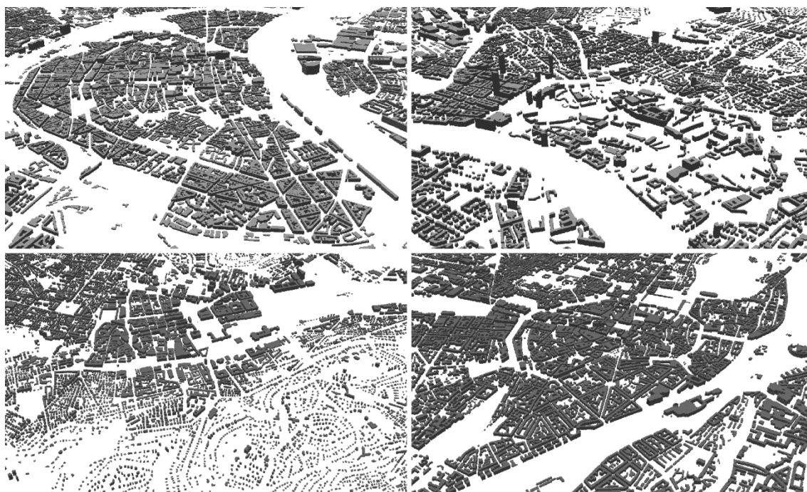
Figure 3. Perspective view of 3D building models derived from space-borne Cartosat-1 height measurements and building footprints from digital topographic maps (top left: Cologne; top right: Frankfurt; bottom left: Stuttgart; bottom right: Munich). Topographic map: © GeoBasis-DE/BKG (2010), cf. [55].
