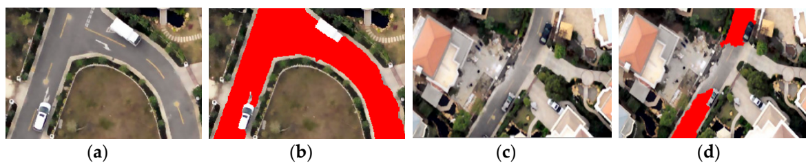
Figure 8. The negative influence of vehicles and Trees. (a) Vehicles; (b) The negative influence of vehicles; (c) The dust, which present different spectra as road; (d) The negative influence of dust.
