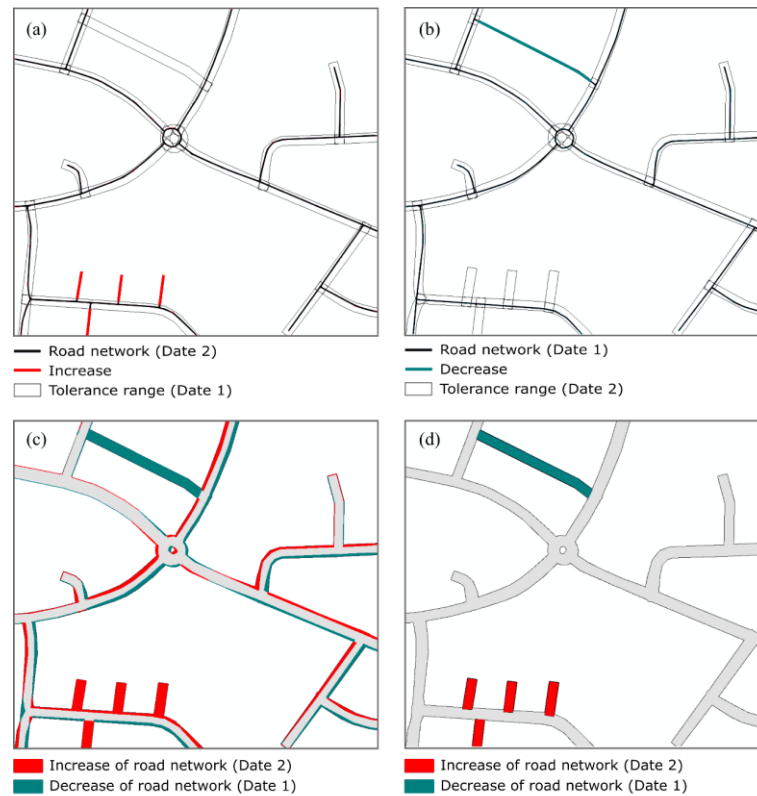
Figure 11. Implementation of tolerance filters regarding line shifting for multi-temporal road network features: (a) increase of road network with a tolerance range of 5 m; (b) decrease of road network with a tolerance range of 5 m; (c) intersection result of uncorrected road network change detection; (d) result of the change detection for the road network with tolerance filters regarding line shifting.
