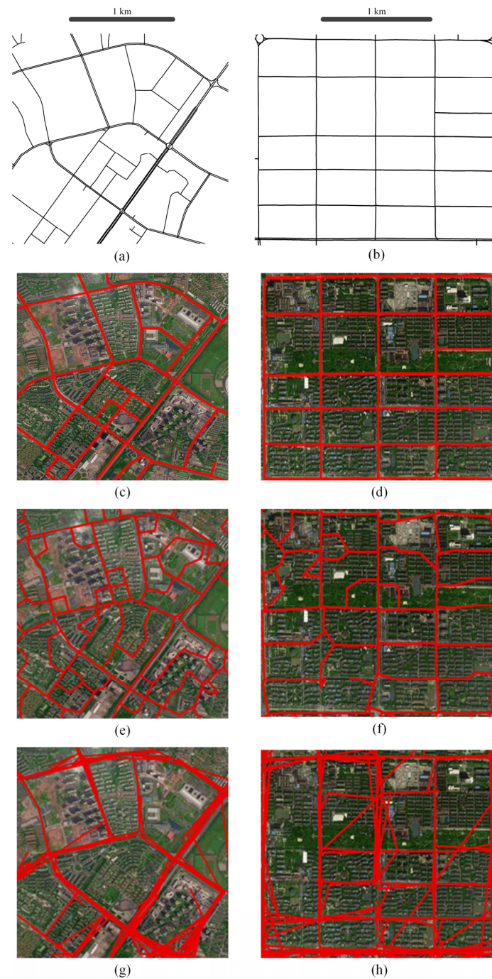
Figure 5. Comparison of road map construction results with benchmark and orthoimage. (a) Zhuankou–benchmark; (b) Qingshan–benchmark; (c) Zhuankou–proposed; (d) Qingshan–proposed; (e) Zhuankou–Ahmed; (f) Qingshan–Ahmed; (g) Zhuankou–Cao; (h) Qingshan–Cao.
