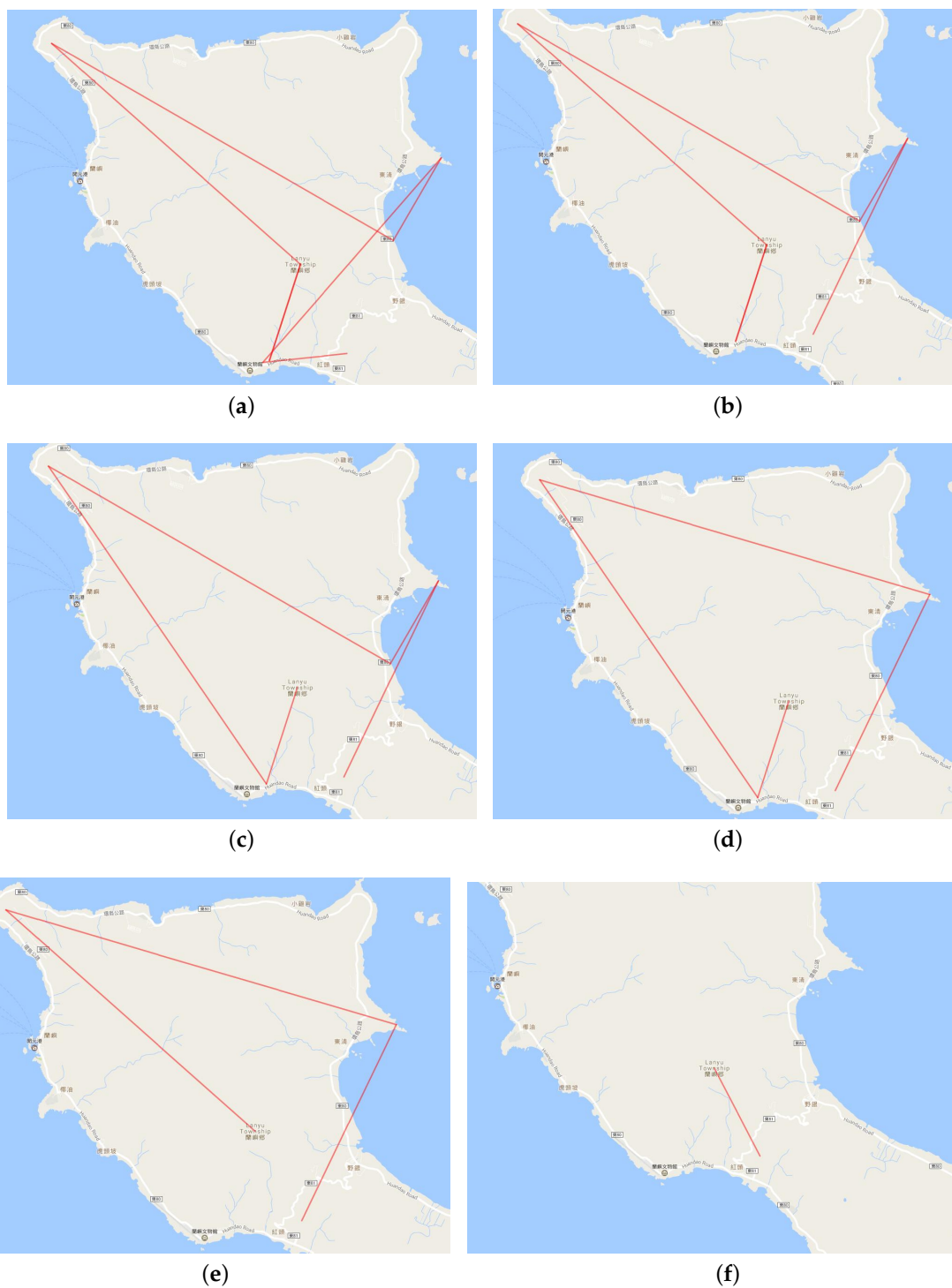
Figure 18. Trajectories between hot site. (a) First compression; (b) second compression; (c) third compression; (d) fourth compression; (e) fifth compression; (f) compression with only one point.
