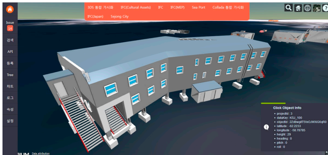
Figure 2. IFC model converted into F4D format and rendered in Mago3D using Cesium.
