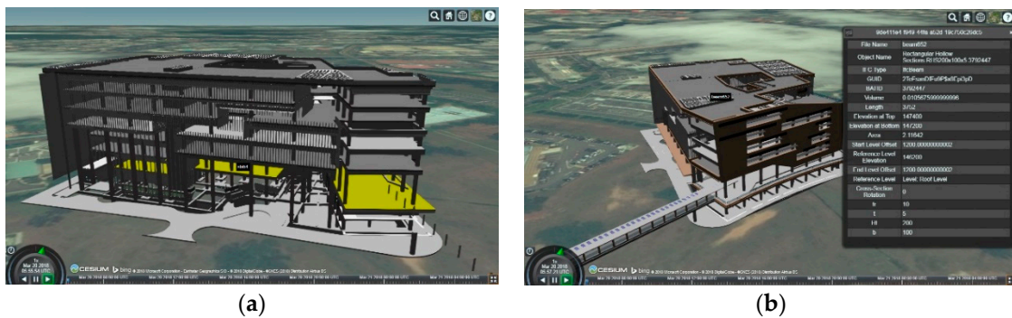
Figure 4. (a) Highlighted individual IFC component in the converted 3D Tiles; (b) query properties for each component from 3D Tiles.
