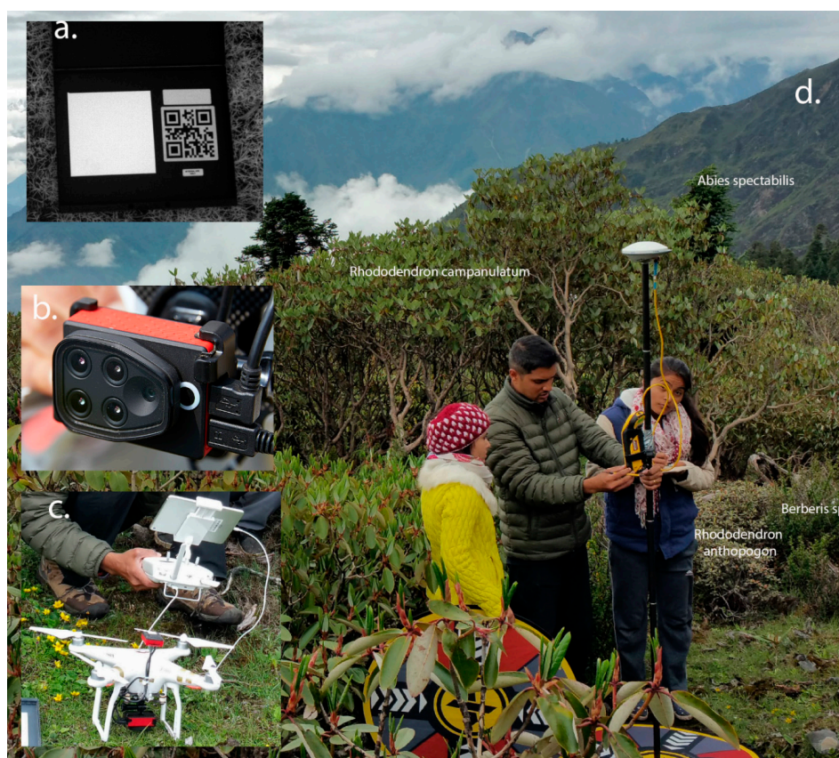
Figure 2. (a) Calibration panel used for estimating surface reflectance; (b) Sequoia camera that acquires images at fixed wavelengths including red-edge and near-infrared; (c) the entire UAS setup with remote and tablet used for mission planning; and (d) setting up ground control points (GCPs) prior to UAS mission in the treeline ecotone in Langtang national park (image date June, 2016). Also labeled are the woody species mapped in this study.
