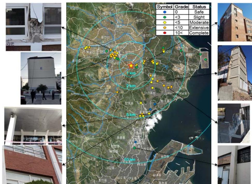
**Figure 8.** Spatial distribution of the earthquake damage categories for majorly damaged buildings and images of buildings.
