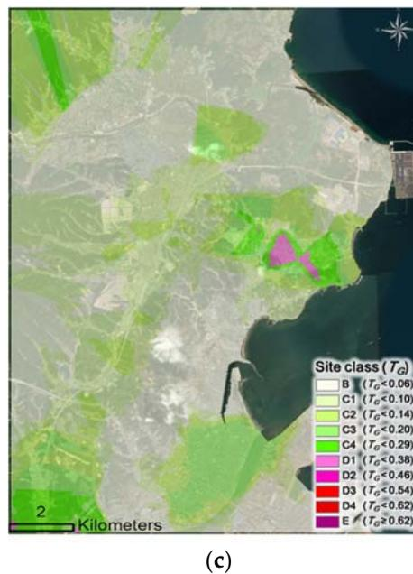
**Figure 6.** Seismic zonation for geotechnical response-parameter-based, site-specific effects: (a)  $H$ ; (b)  $V_{S30}$ ; (c)  $T_G$ .
