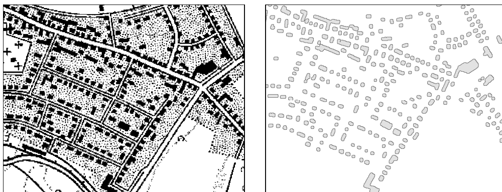
Figure 2. Original binarized map images (left, black–foreground, white–background) and the retrieved building footprints (TK25 © LVerGeo 2014).
