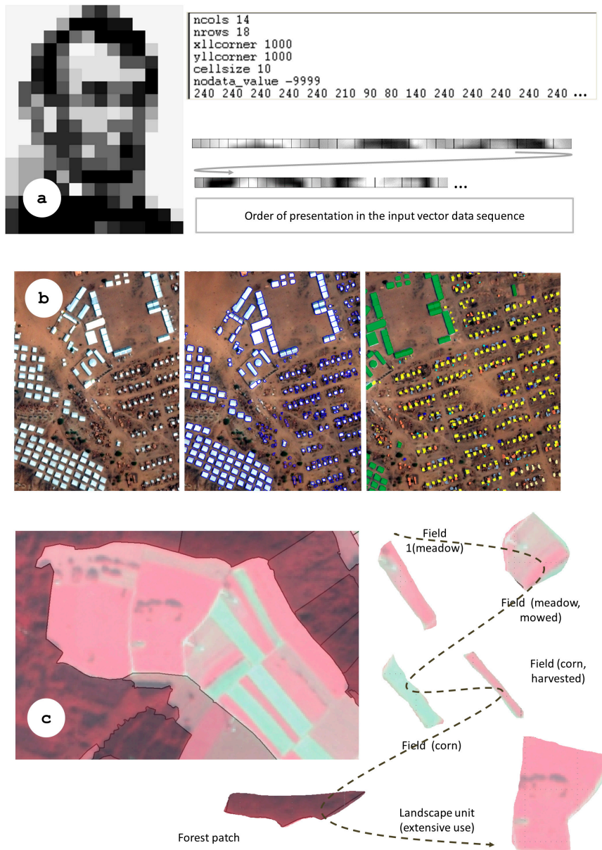
Figure 2. From 1D to 2D image analysis, a recognizable (pixelated) 2D image (a) of Abraham Lincon (at left) is transformed into the 1D vector data stream shown on the right. This 1D vector data stream, either pixel-based or local window-based, means nothing to a human photointerpreter. This (out-of-context) 1D vector data stream is what the inductive classifier actually ‘sees’ when analysing the (2D) image at left. (b) Similarly, the linear sequence of segmentation and classification—often applied in standard GEOBIA workflows—may suffice for singular feature extraction tasks such as classifying dwellings in a refugee camp, but falls short (c) when modelling ‘composite objects’ such as ecologically relevant complexes, e.g. a mixed-arable land as shown (bottom-right).
